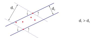
The lines can be rotated up to where one of them intersects a new point. When one line contains two points and the other contains one point, the lines are said to comprise a *lock*, and the distance between them is called a *lock value*.
