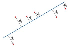
As the fit between the plane and the points gets better, the quantity  $D = d_1^2 + d_2^2 + \cdots + d_n^2$  gets smaller. Usually one *best fit* plane exists for which D is as small as possible. Unfortunately, flatness is only approximately equal to the minimum distance between sandwiching planes parallel to this best fit plane. To see this, consider the four points below to the left, and the six points below to the right.
