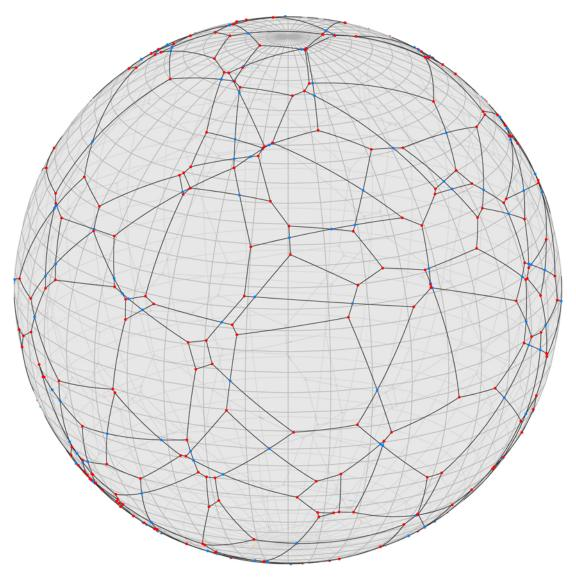
Traversal of the lock network allows for a rapid and efficient evaluation of every single lock value. The minimum of these values is the flatness of the original point set.
