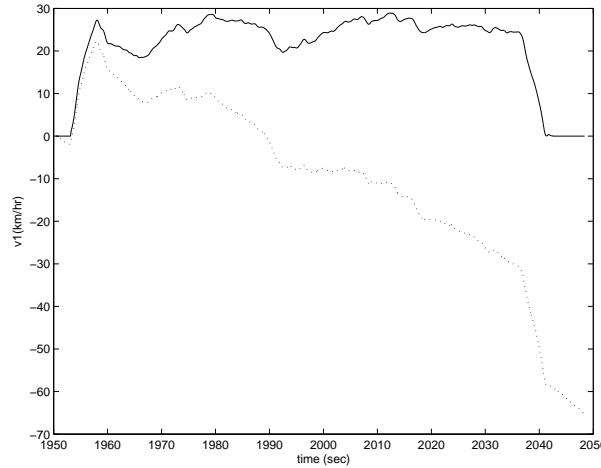
Figure 11: Velocity profile constructed from data in Figures 10 and 9. The dotted line is our initial result, obtained by integrating the filtered signal from the forward pointing accelerometer. We know that the motorcycle is stationary at the beginning and end of an interval of forward motion, so we apply a linear adjustment to the dotted line to get the reasonable velocity signal shown as a solid line. We also know that the motorcycle is at rest before and after the middle part of the test run, so we set the velocity to zero during these periods.
